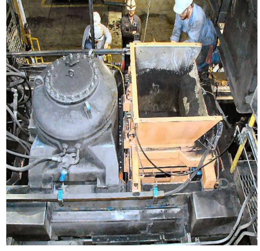
heavy-duty industrial AC gear-motors. Each motor is controlled by it's own frequency inverter drive. This provides a wide speed range for each spindle with full torque. The unique ESI system also provides individual rotation and speed selection capability for each spindle. There
